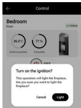
Fig. 10.2 Screen asking the user to confirm whether they want to light the fireplace
