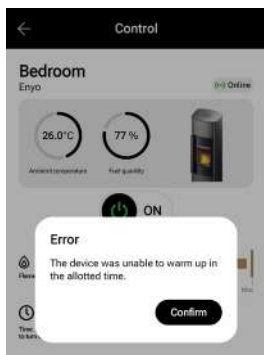
Fig. 15.4 Message indicating improper heating of the device
