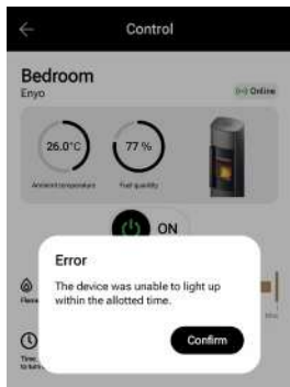
Fig. 15.2 Message indicating that ignition is not possible due to an insufficient fuel level
