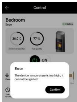
Fig. 15.1 Message indicating that ignition is not possible because the device temperature is too high
