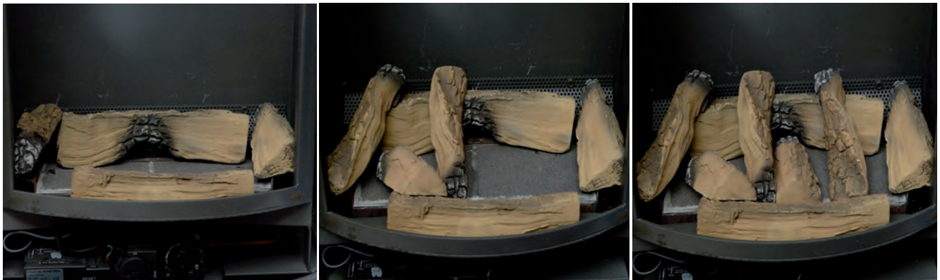
Arranging the log set for natural gas.
